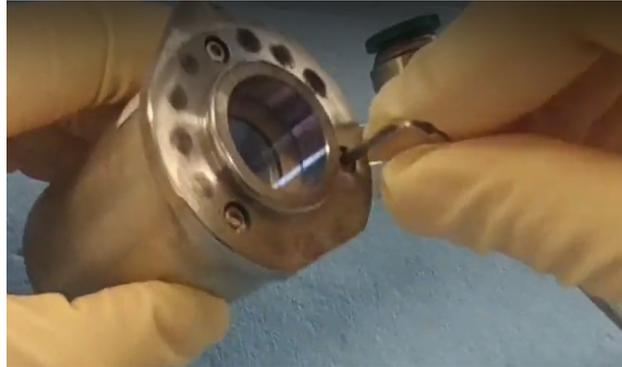
3. Remove the window by shaking the nozzle above the lens paper. If the window does not come out, gently extract it by holding it on the edges.
