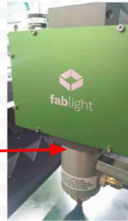
Face flat edge to green cover side of cutting head. Ensure nozzle is sitting properly and securely back in cutting head by giving it a test tug and twist, there should be no play.
