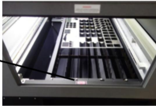
On the cutting head is this label, warning about exposure from the cutting head aperture.
