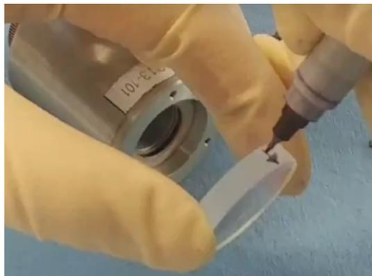
5. Open the replacement window package. Wearing gloves, grasp only the EDGES of the window to lift it out of its case. Do not touch the surfaces (top or bottom) of the window.
