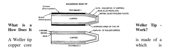
electro-plated with iron to extend the life time of the tip. The non-working end of the tip is plated with nickel for protection against corrosion and then chrome plated to prevent the solder from adhering except where desired. The wettable part is tin covered.
