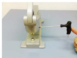
The yellow brass cylinder has a slight conical shape. If you loosen the headless Allen key screw in the grey aluminium body, you can change the position of the upper tool by turning the cylinder.
