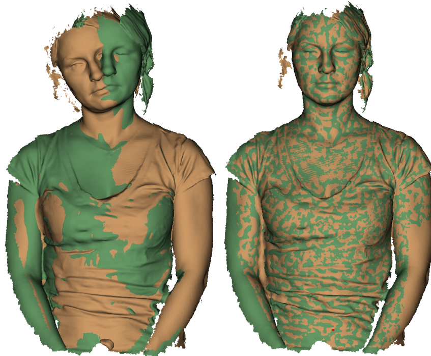
Figure 84: Two models after rigid (left) and nonrigid alignment (right).
